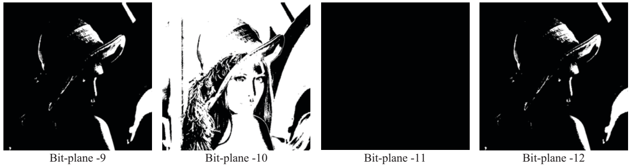
Fig. 2. Image bit-plane decomposition using the Phi number system (base- \phi ) with numerals \{0,1\} .
